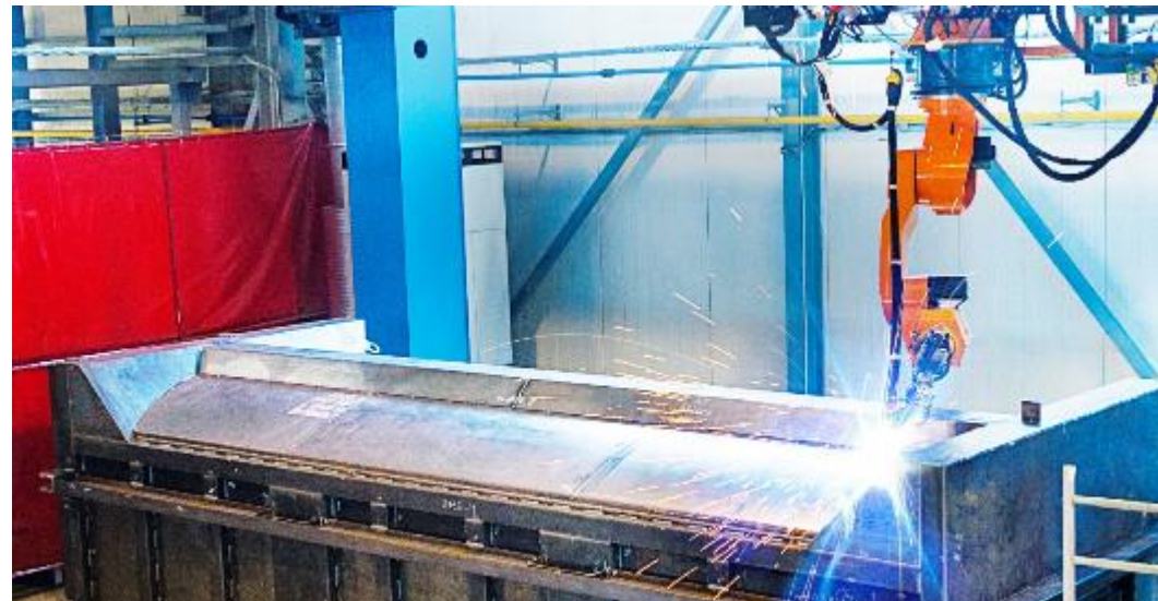
A robot welding a waste container at MariComp Tallinn plant.
